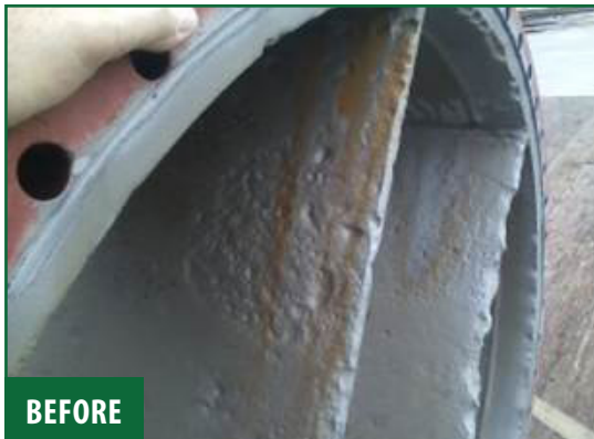
Pitted and worn steel rebuilt with Novocoat EP3920 Machinable Grade .
