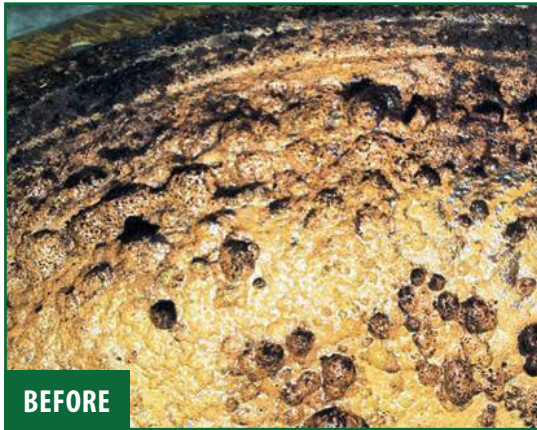
Heat exchanger floating head before and after pits in steel were filled using Novocoat EP3920 Machinable Grade . Novocoat SC5400 applied as topcoat.
