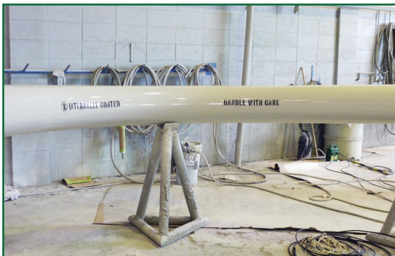
Novocoat SC2200 Rapid Set Pipe Coating applied on outside. Novocoat SC3300 Series applied inside.
