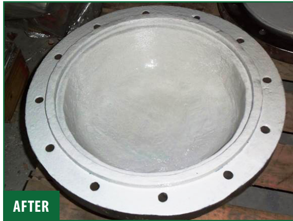
Heat exchanger floating head before and after pits in steel were filled using Novocoat EP3920 Machinable Grade . Novocoat SC5400 applied as topcoat.
